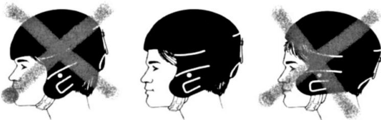
The helmet must not be seated on the back of the head, leaving the forehead unprotected. It must also not be pulled down too much over the forehead, as this could impair visibility.
